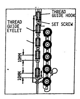
THE RELEASE WEDGE MUST REACT EARLIER THAN THE THREAD TRIMMER'S OPERATION, WHEN ADJUSTING, LOOSENING THE SET SCREW, SETTING THE PROPER POSITION OF RELEASE WEDGE. IN THE MEANTIME, PLEASE MAKE SURE THE RELEASE WEDGE CAN PUSH TENSION DISC COMPLETE APART AND ALSO CAN RETREAT COMPELELY (CAN NOT INTERFERENCE WITH TENSION DISC.)
